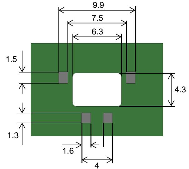
Card edge design for converter board
