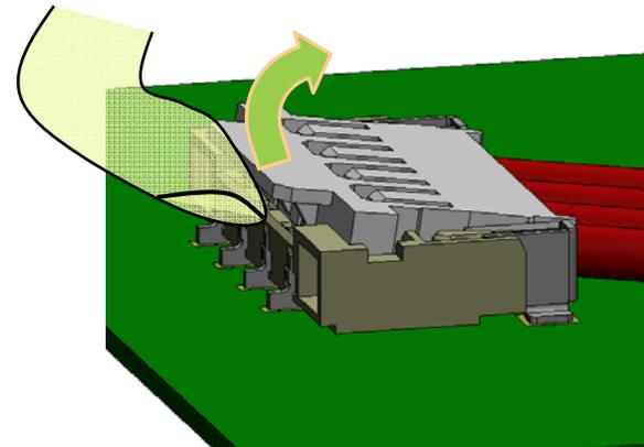
Pull up on the front side of the plug. Pulling up on the cable side will not disconnect the plug.
