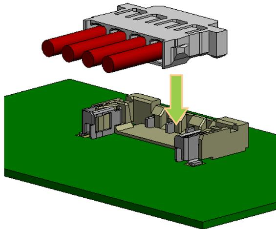
Insert the plug from above and push down until the plug is flush with the top of the receptacle.
