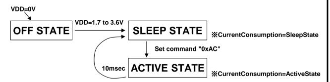
OFF STATE···The sensor is not active when VDD is disabled.
